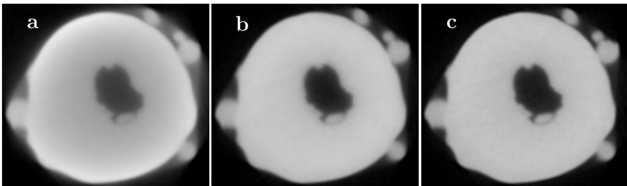
Figure 1: Horizontal slices through a reconstructed volume: a) without any correction, b) modelling attenuation as photoelectric ( $K_2 = 0$  in Eq (1)), c) assuming a constant atomic number of material ( $Z = \text{const}$ ).
