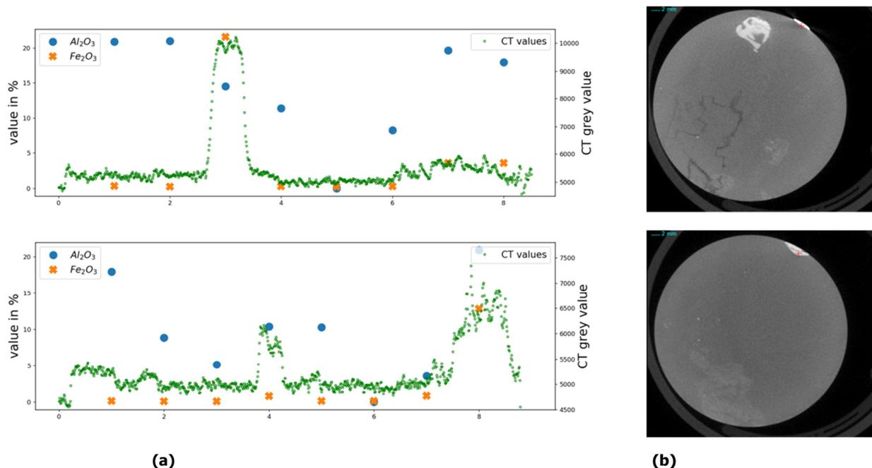
**Figure 1:** (a) Concentration of  $\text{Al}_2\text{O}_3$  (o) and  $\text{Fe}_2\text{O}_3$  (x) determined by means of XRF and corresponding grey value profile (spots) extracted from the reconstructed CT volume. (b) Reconstructed CT slice corresponding to measurement point 3 of scan 1 (bottom) and slice showing an inclusion which is not detectable with XRF or LIBS techniques (top). The zinc foil on the surface is intersected.
