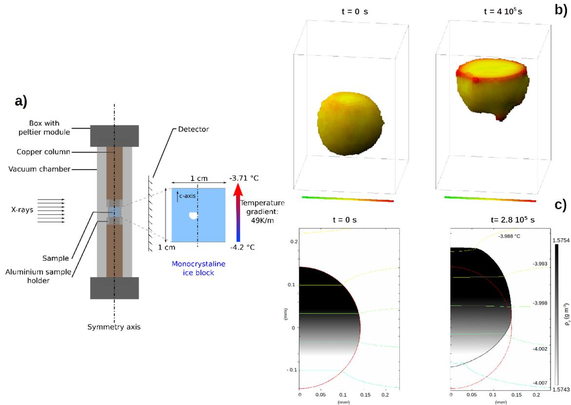
**Figure 1:** (a) Scheme of the experimental setup. (b) 3D images of the cavity obtained with microtomography, colors represent mean curvature of the interface. (c) Simulation results of phase-field modeling. Black and red isolines are interface positions at  $t = 0$  and simulated time respectively. Coloured contours are temperature isolines. Grey levels represent water vapor density in the air space.
