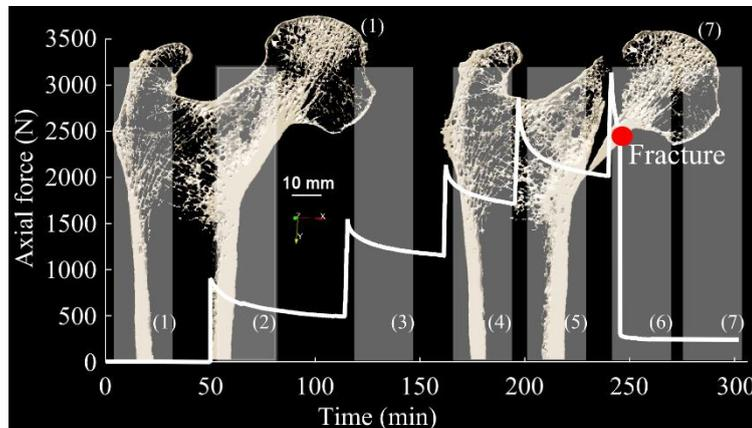
**Figure 1:** Load time history (white line), scanning time (gray bars) and 2 mm-thick 3D synchrotron micro-CT volumes (in yellow) of a femur unloaded (1) and once fractured (7).
